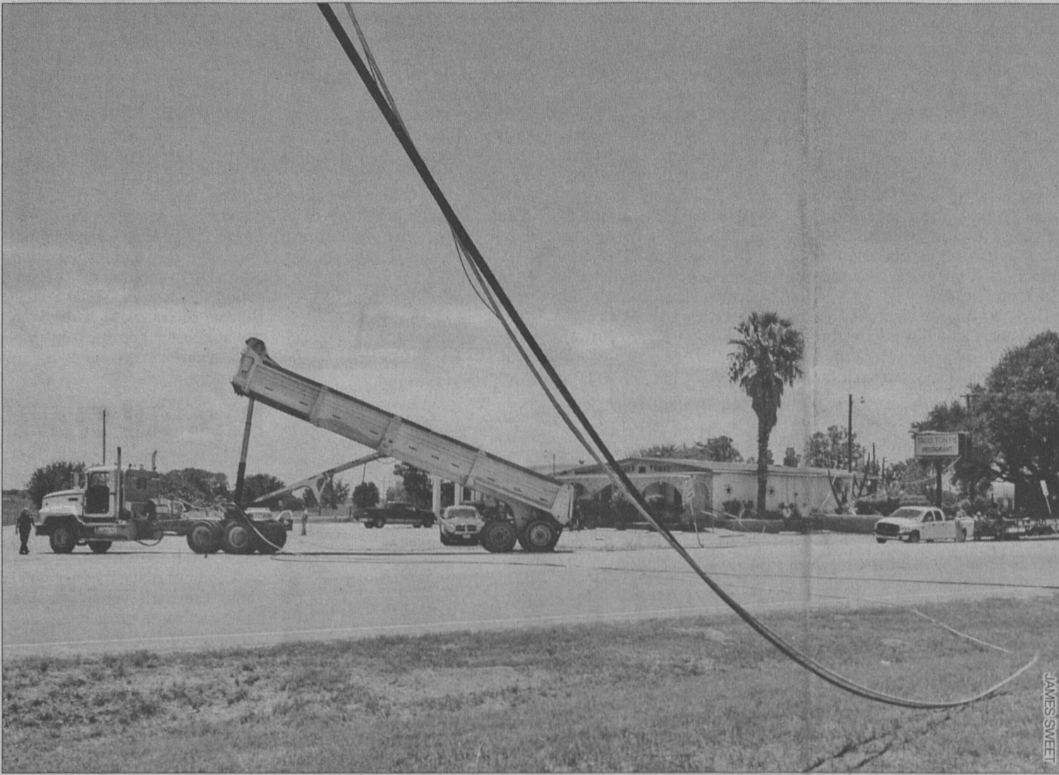
Pictured above is an 18-Wheeler that took out power lines near Taco Tony's Monday at about 1 p.m. The driver was apparently driving with the bucket of the truck upright when it struck an overhead power line.
